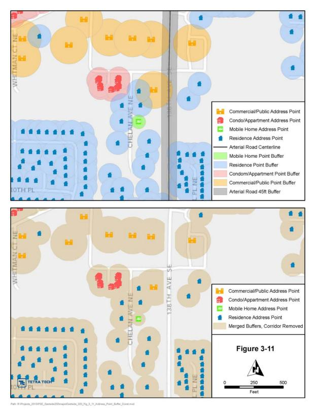
Figure 3-11. Structure Buffer Process
