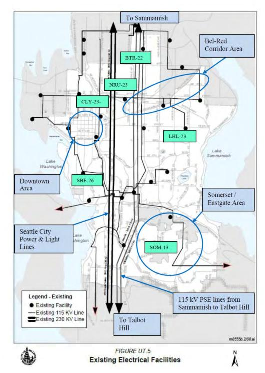
Figure 30. Existing Transmission Facilities around the City of Bellevue
