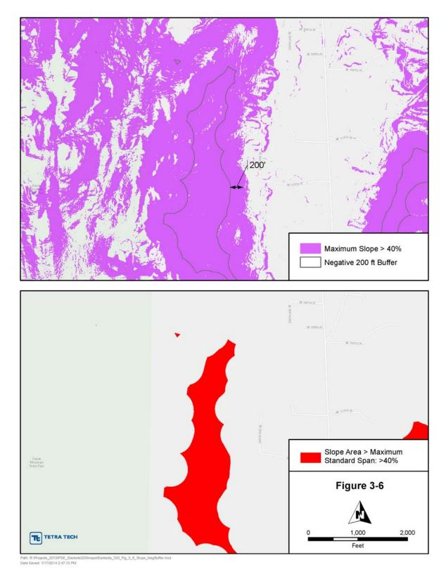
Figure 3-6. How Unspanable Slope Is Derived
