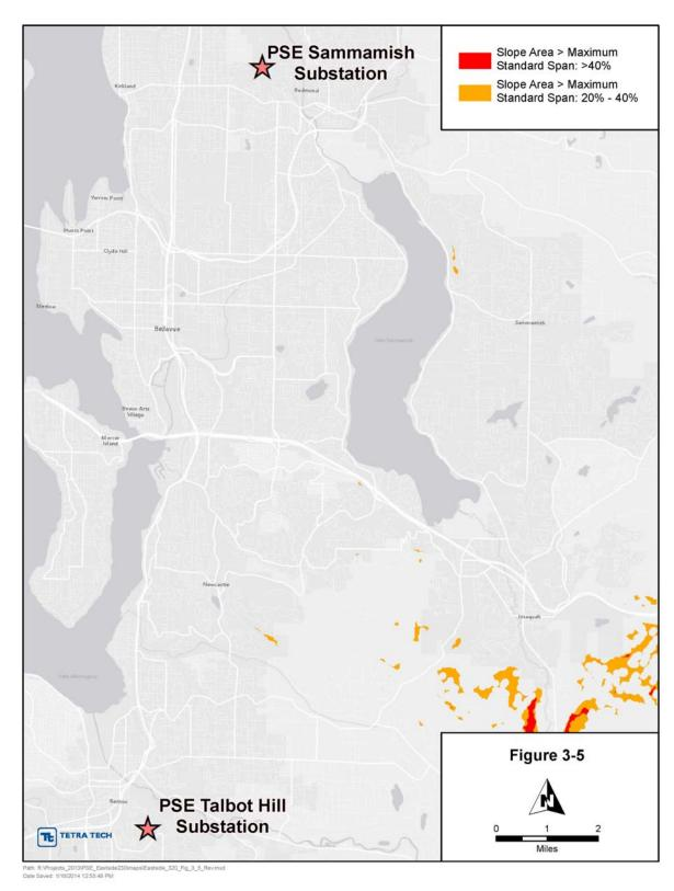
Figure 3-5. Unspanable Slope
