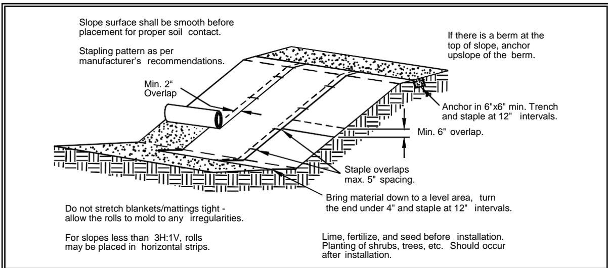
**Figure 4.1.4 – Slope Installation**
